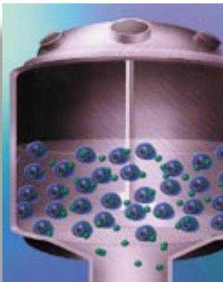
To foster cellular replication and production of rhBMP-2, they are transferred to a bioreactor, a computer-controlled, closed-system environment where large-scale production of rhBMP-2 begins. After a growth period of about three days, the recombinant cells are filtered away from the rhBMP-2 containing medium and discarded. The rhBMP-2 moves on to the purification process.
