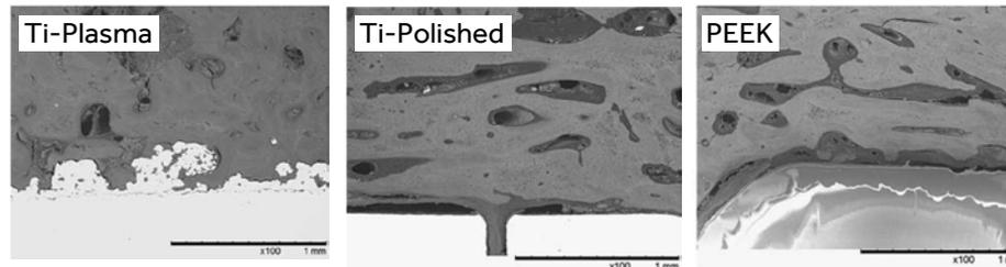
SEM of implants in sheep spine model. Ti-Plasma treated surfaces had greater proportion of surface in contact with bone with less direct fibrous tissue contact than Ti-Polished surfaces and PEEK.
