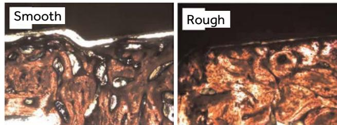
Histology section of smooth and rough Ti6Al4V pedicle screws in sheep spine. Smooth Ti6Al4V were covered by fibrous tissues whereas rough Ti6Al4V showed more direct bone contact and produced mineralized matrix.
