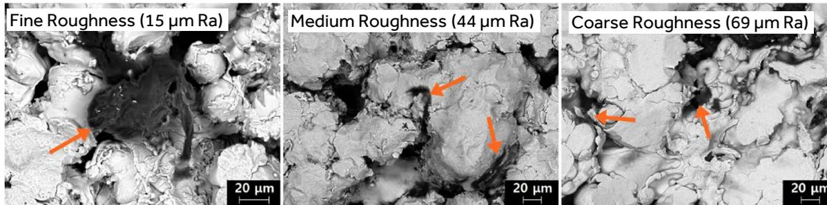
Environmental SEM of hMSCs cultured on different roughness CPTi-coated PEEK. Fine roughness resulted in stronger adhesion and greater pseudopodia extensions (arrows).
