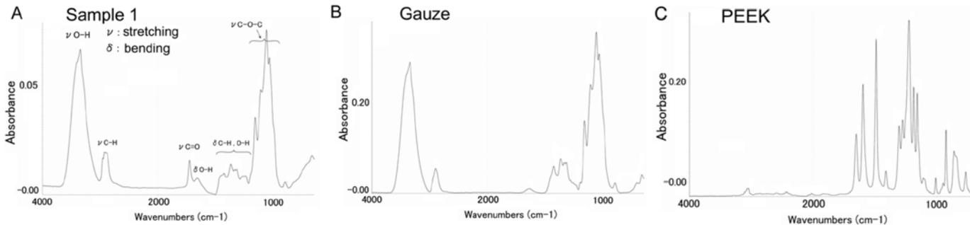
FTIR Spectroscopy on foreign particles (sample 1) at vertebral osteolytic defect suggests it is derived from cotton gauze.
